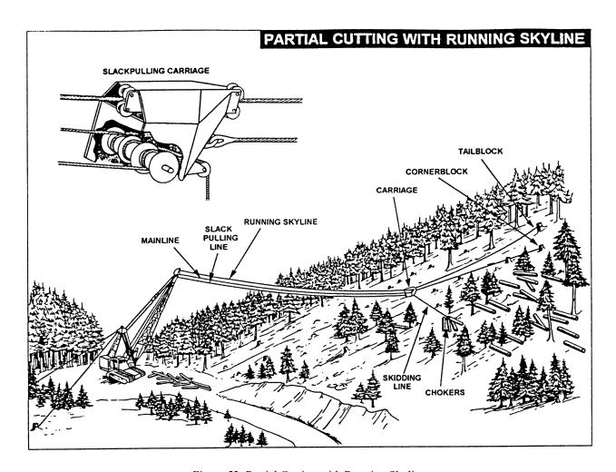
Figure 53: Partial Cutting with Running Skyline
