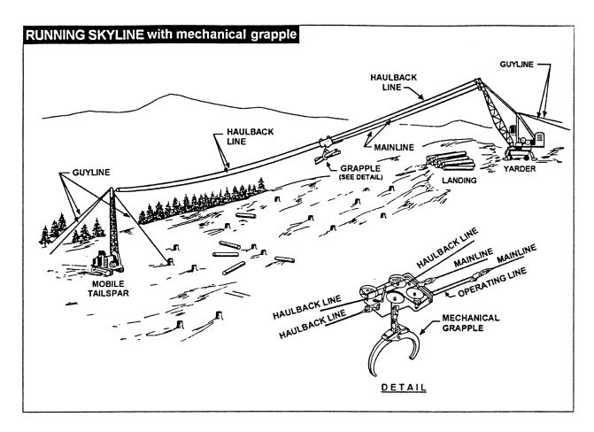
Figure 55: Running Skyline with Mechanical Grapple
