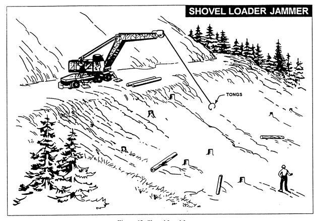
Figure 43: Shovel Load Jammer
