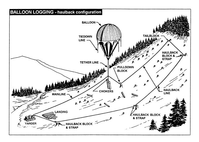
Figure 58: Balloon Logging - Haulback Configuration
